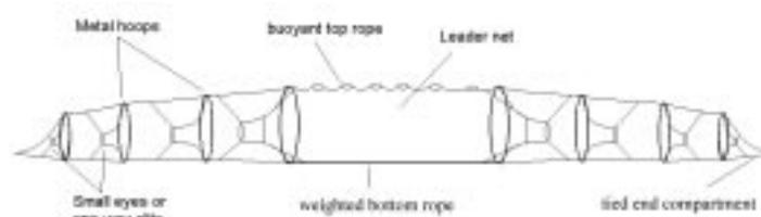
Figure 1 Fyke net
