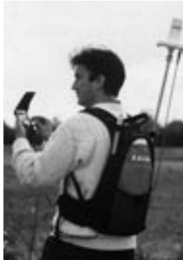
**Figure 2** Typical dGPS rover configuration<sup>3</sup>
