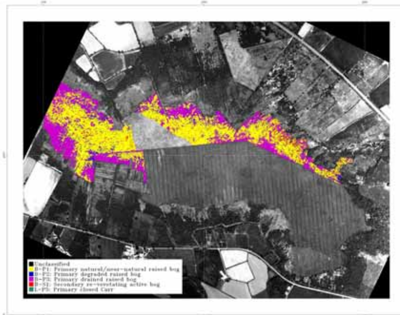
Figure 36. Maximum likelihood classification of the undisturbed areas of Ballynahone Bog
