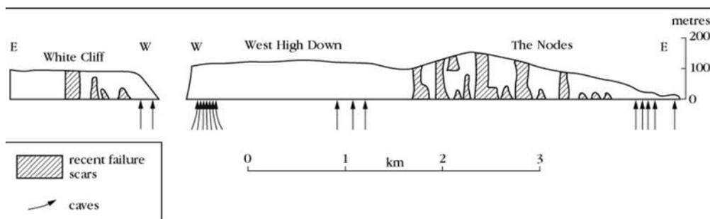
Figure 4.21: Cliff-face failures west of Freshwater Bay. (Based on British Gas aerial survey, February 1996.)
