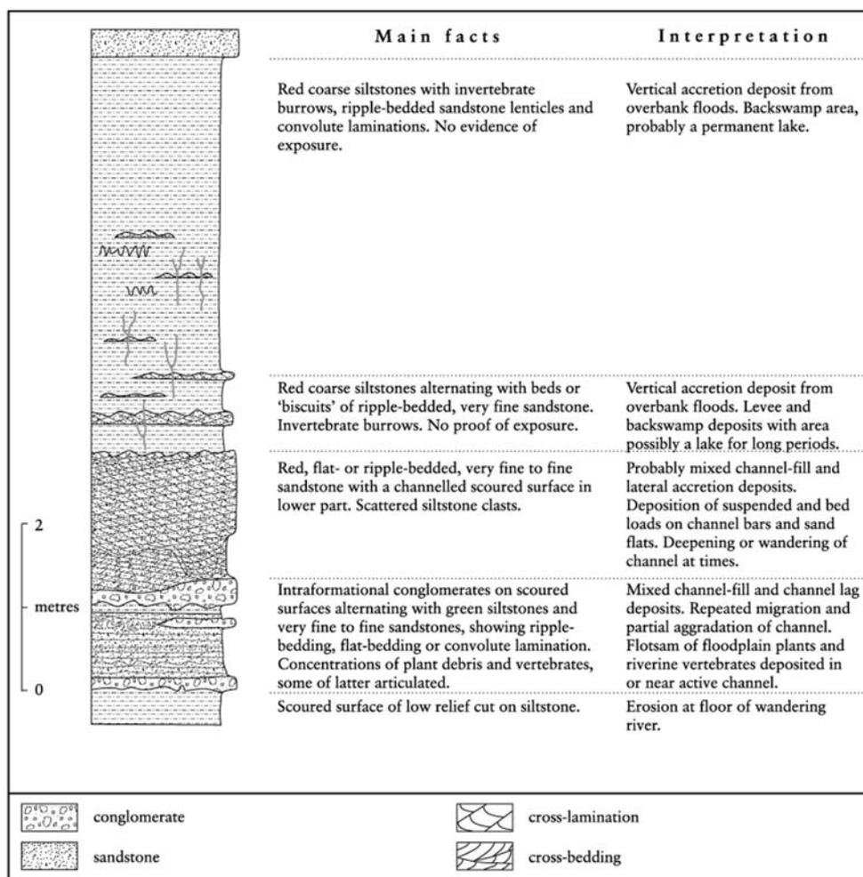
Figure 4.13: The succession at Cwm Mill, Abergavenny (after Allen, 1964).
